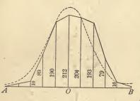
slight preponderance of shots below the middle, and there is reason to believe that this is due to a constant error of gravitation not entirely eliminated in the sighting of the gun. If this series of shots were to be repeated again under exactly similar condi-
